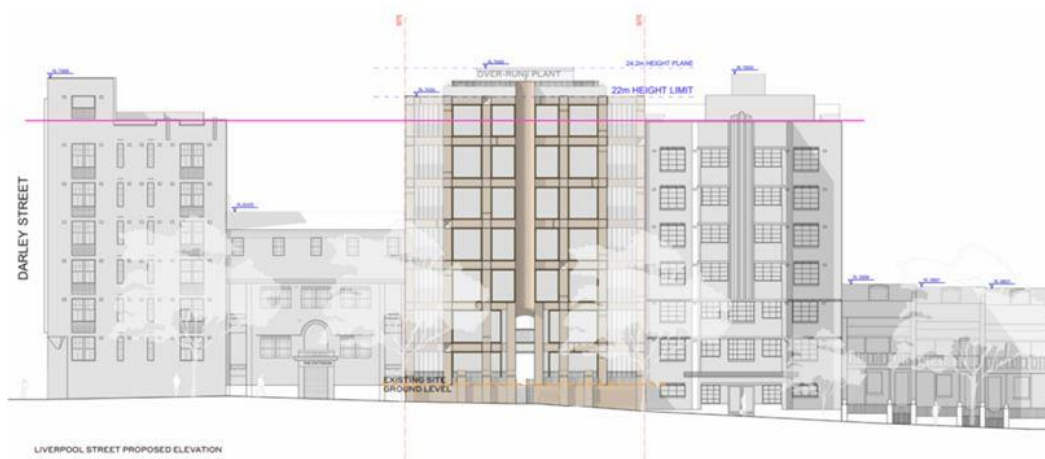
Figure 36: The Liverpool elevation drawing extract depicting the context of the original proposal along the southern side of the street, with the parapet line of the tallest existing buildings in the street outlined in pink
